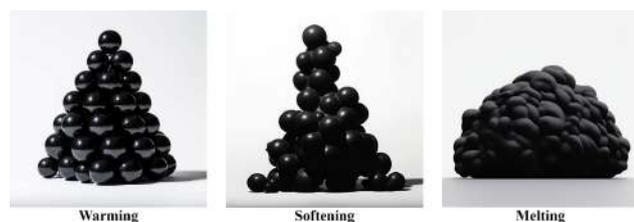
Fig. 2. Schematic illustration of the fusing stages of toner in electrophotographic printing.
